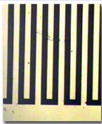
Optical image of gold fingers on a glass substrate.
