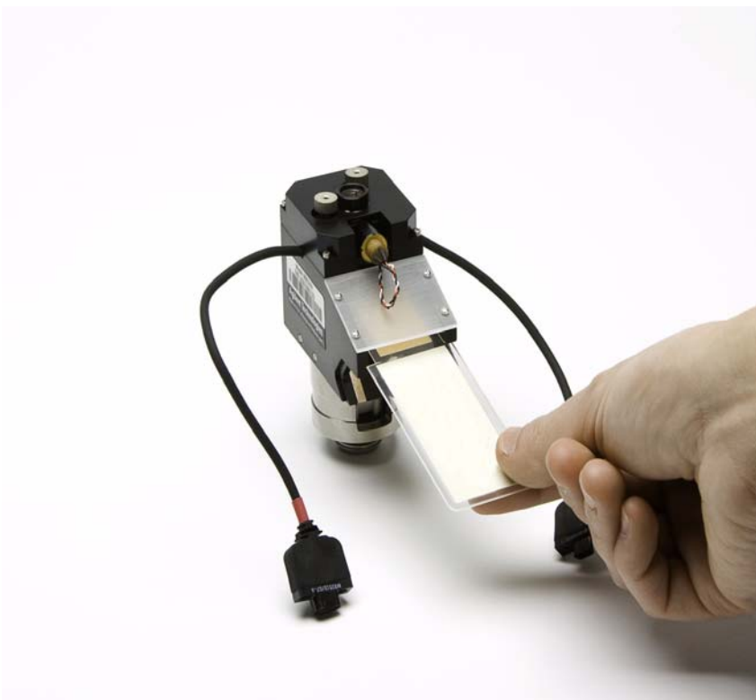
Figure 53 Coarse laser alignment for IR scanners using sensor card
