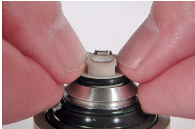
Figure 33 Applying even, vertical pressure at the edges to insert the nose assembly.
