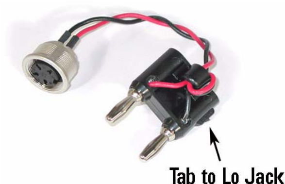
Figure 134 Tab side of Cable 3 must be inserted into the Lo jack.
