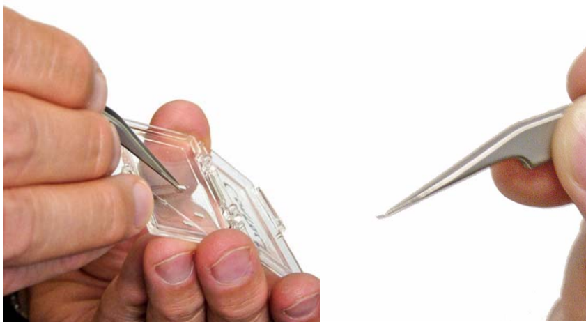
Figure 39 Holding the tweezers as shown, remove a probe from the protective case
