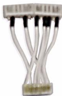
Figure 131 Hot MAC sample stage Y cable.
