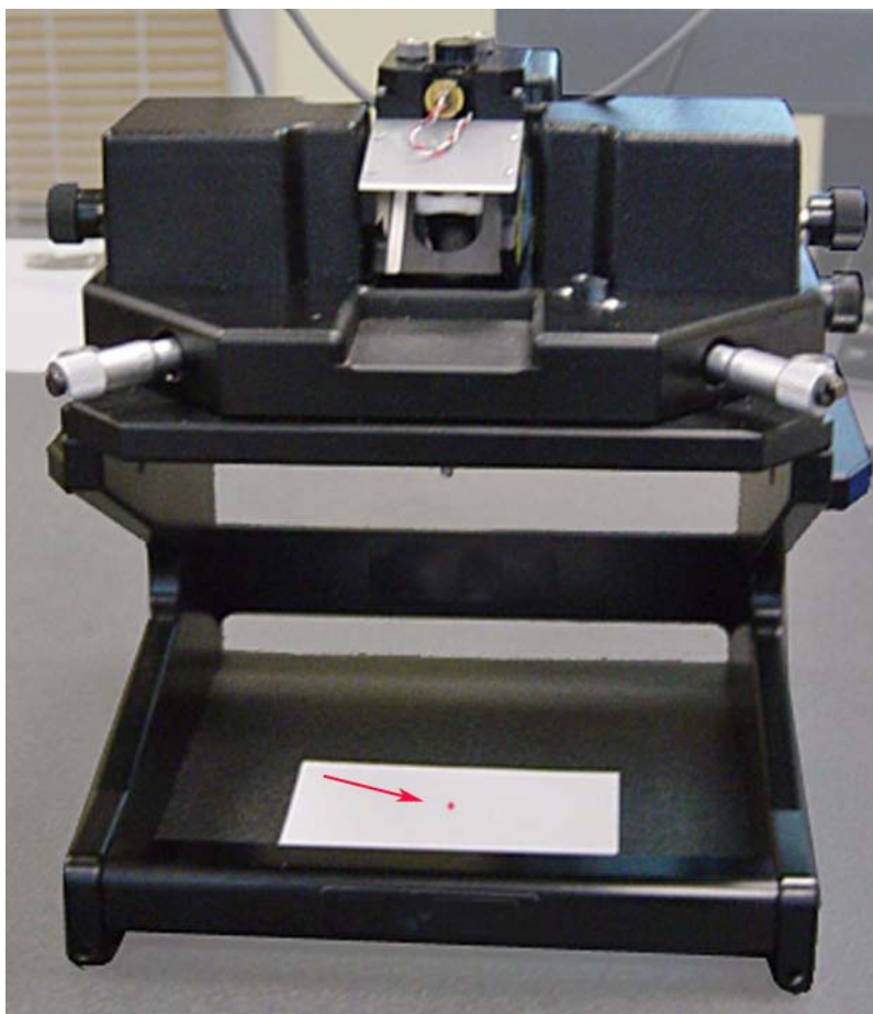
Figure 46 Aligning laser spot over white paper.
