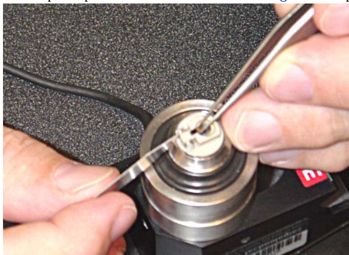
Figure 40 Hold back the retaining spring while placing the probe
