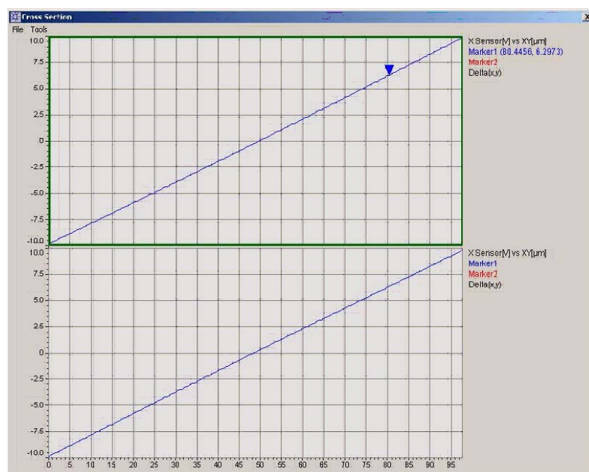
Figure 108 Cross-section after Offset and Gain values optimized
