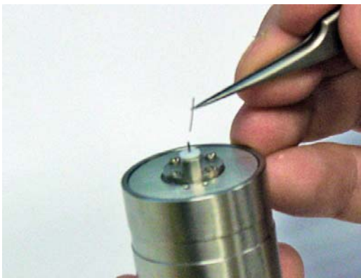
Figure 82 Inserting STM tip wire in scanner
